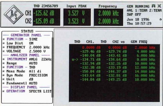
Fig. 11: Complete measured-value tables can be output for all functions
